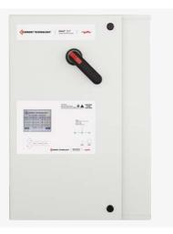
Select® SL3™ suppression filter systems feature selenium-enhanced surge protection along with a powerful failure-free ISM™ (Integrated Suppression Module). The ISM™ contains individual thermally fused and protected MOVs, surge-rated copper busing, robust filtering and advanced remote communications capabilities. Additionally, the SL3's selenium-enhanced seamless technology design ensures maximum performance and a dramatically extended product life.
